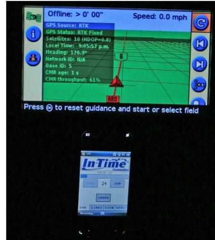
In all cases, wireless access of RTK correction signals over a cell phone allow more freedom for the end-user, less signal loss, increased productivity, and lower operating cost. Operating 15-20 miles from the base station is no problem with this system<sup>3</sup>.
